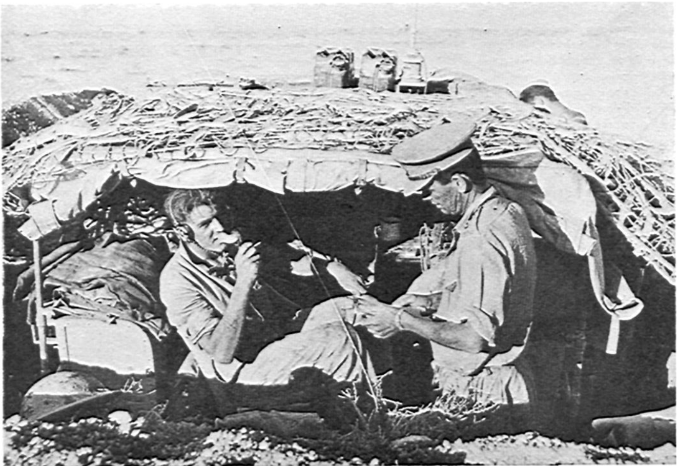
Communications and other vehicles are often well dug in. This protects their running gear, and the lower silhouette reduces chances of discovery.
