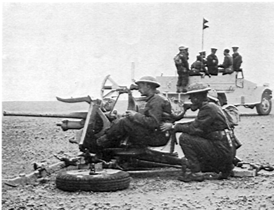
Shield of the 2-pounder can be lowered for better visibility, when necessary.
