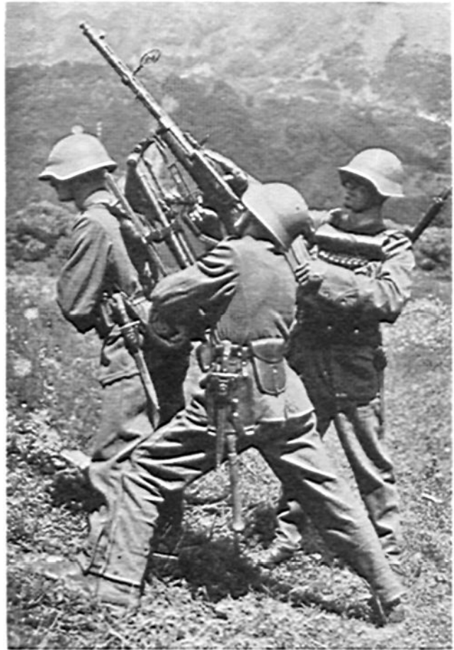
The Swiss 7.54-mm. light machine gun is air-cooled and recoil-operated, uses a 30-round magazine and either bipod or tripod mount. The gun alone weighs 18¾ pounds, and the respective mounts 4½ and 23½ pounds. Rate of fire: 450 rounds per minute. Ranges: maximum 4900 yards: maximum effective 1600 yards. (Photo Widmer, Wallenstadt.)
