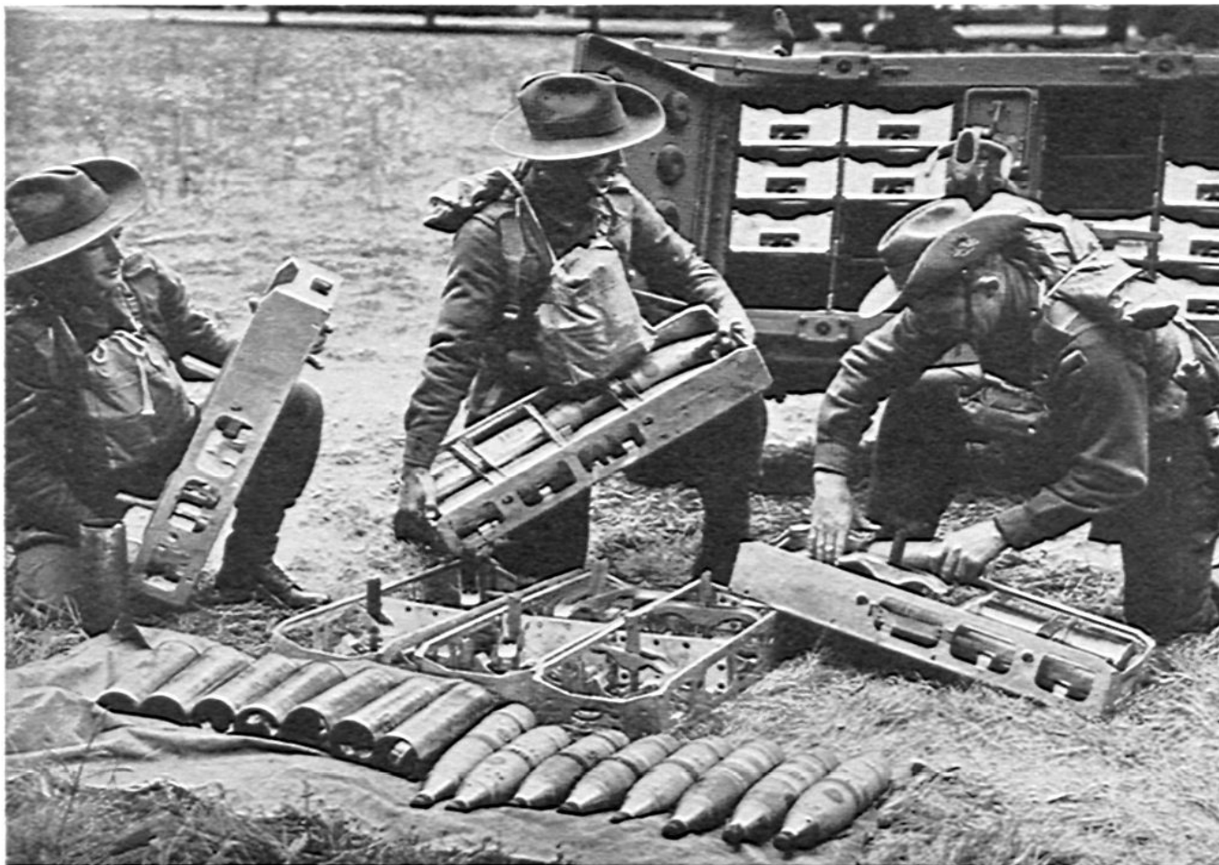
Trailer carries 32 rounds of separate-loading ammunition, with two complete rounds per tray. On end of the metal cartridges can be seen handle of plug which is pulled out for removal of undesired powder increments, then replaced. Spare parts are carried in the central space; below pintle for towing the piece is a spare tray, also filled with spare parts. AP projectiles are carried separately, and are in addition to the regular complement of complete rounds as the same cartridges can be used for them; usually they are strapped on top of the trailer.
