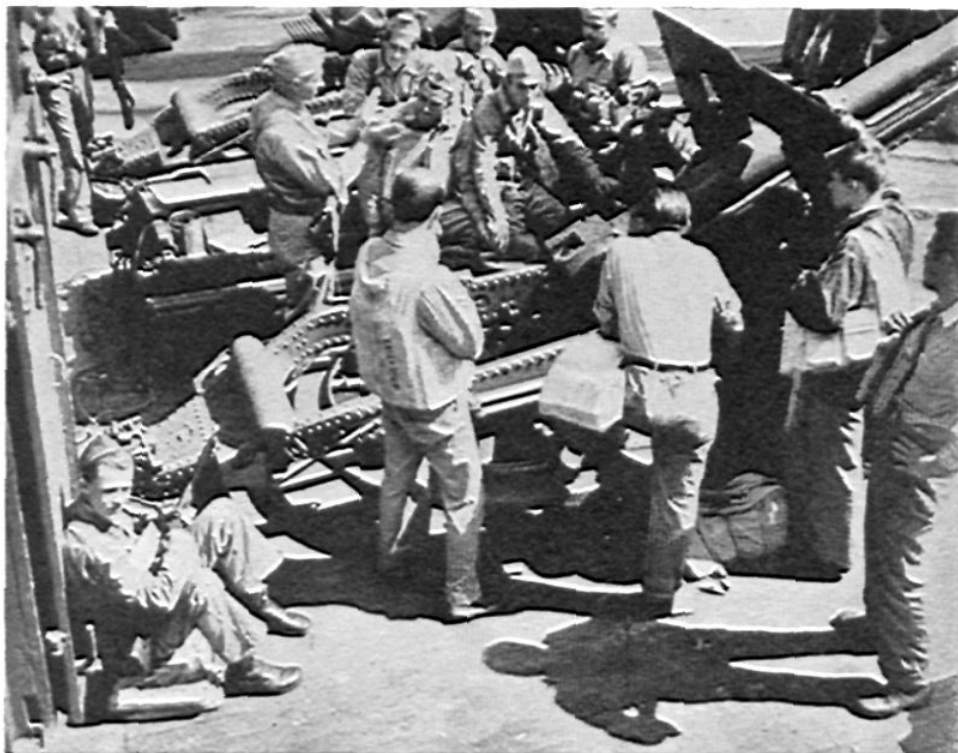
These troops of ours, bound for New Caledonia, are becoming familiar with the 25-pounder. Notice how the flat portion of the trail furnishes an alternative place in which to carry the firing platform; this is what causes the arched appearance of the trail.
