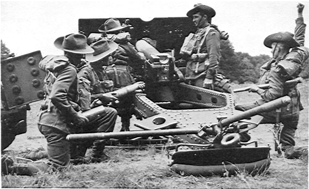
Piece loaded, ready to fire, with crew ready for the next round. Note spade box in place, to prevent spade from digging in; this is a necessary precaution if maximum use is to be made of the rapid traverse afforded by the platform.
