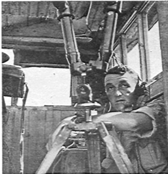
Objective lenses of this BC 'scope are fitted with short sun-shades.
