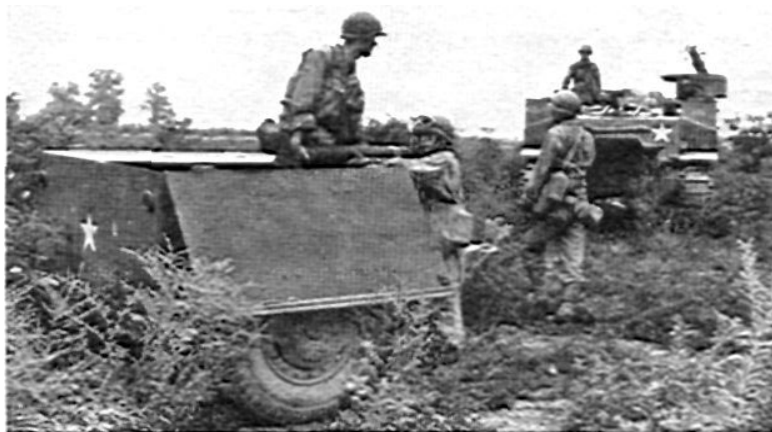
Pass the ammunition.—The M7 is largely self-sufficient, for there is room in the vehicle for necessary crew and equipment. A good load of ammunition is carried in an armored trailer and so, if the M7 gets within range of the enemy, it has all it needs to go into action. Here men are unloading shells from the trailer and carrying them to the M7, where No. 4 cannoner will prepare the charge and hand the rounds up over the side to No. 3, who sets the fuze.
