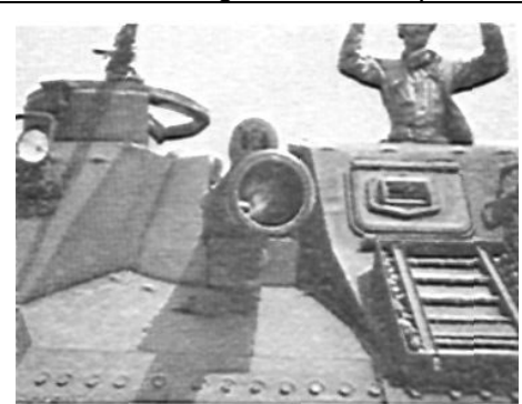
Armored artillery is still artillery. Whatever the means of transporting it to the firing position, it is still a 105-mm howitzer that delivers the punch, Armor and self-propelled mount merely enable it to take up positions where it will be most effective in support of tanks and armored infantry.
