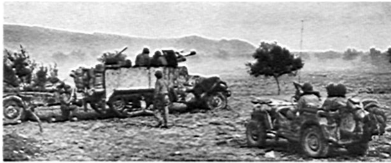
Some half-tracks in North Africa were equipped with 105s instead of standard 75s. Their heavier firepower was invaluable, and their carriages stood up surprisingly well under the heavier recoil.
