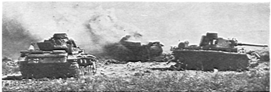
. . . results like this, wherein a battery of 6-pdrs. knocked out 3 of the newly modified Pz. Kw. Ills in short order. The Nazis have been mounting larger caliber guns with higher muzzle velocities on most tank models; this combination makes it imperative that our AT guns NOT open fire (or otherwise disclose themselves) prematurely.
