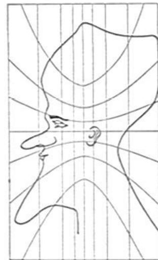
Fig. 4—Man's head plotted on a gnomonic projection
