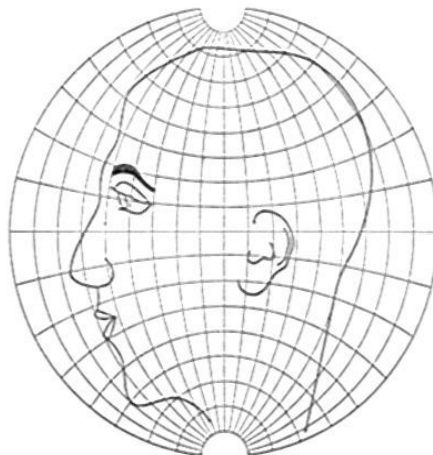
Fig. 6—Man's head plotted on a polyconic projection
