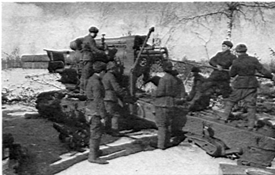
Russia's 21-cm. howitzer has well proved itself in the present war. Tracks give it greater flotation, and higher degree of stability in firing, than would wheels. Small carts are used to move ammunition about the position: when hoisted, they form loading trays.
