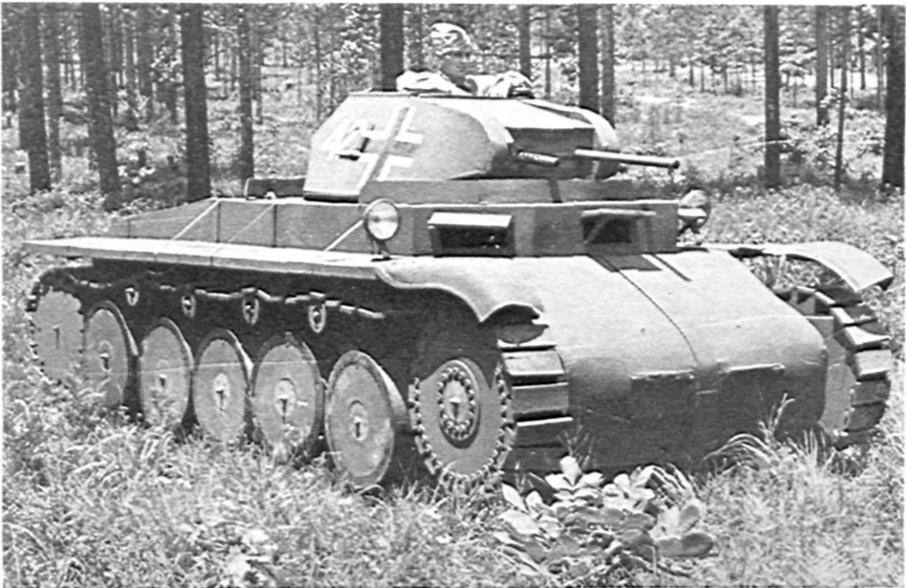
German Pz. Kw. II, now used mostly for reconnaissance, liaison, and flame throwing. This model is built over a jeep, for realistic movement.
