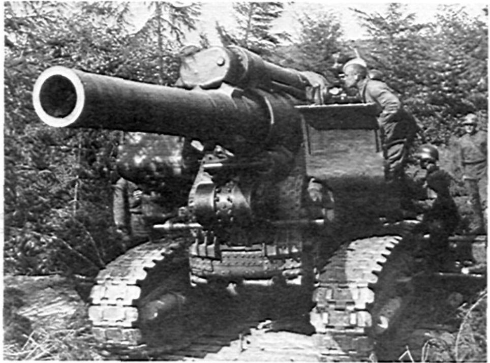
Russia's 210-mm. howitzer is ready to go as soon as uncoupled (Sovfoto)
