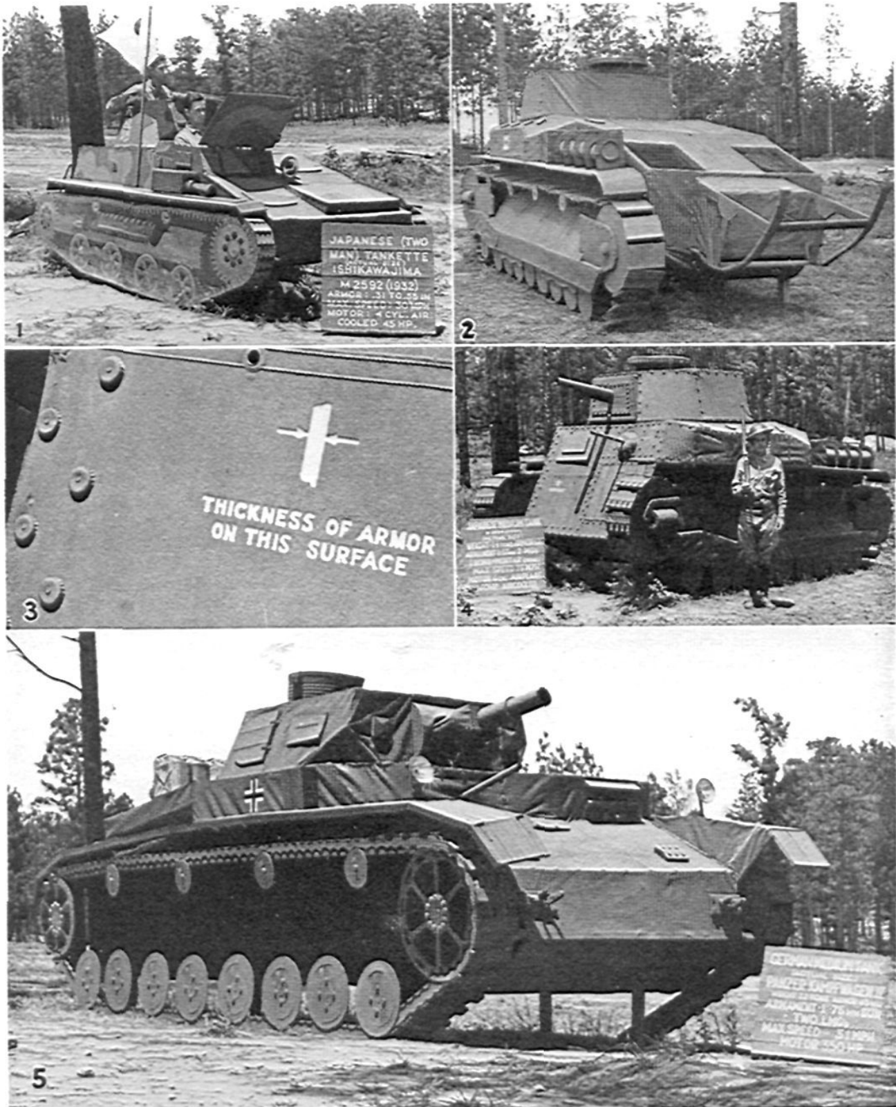
Figure 1—See board for description. All photographs are by Lt. R. B. Rigg except Figure 2, which is a U. S. Army Air Corps photograph. Figure 2—Rear view of Japanese medium tank M2594 (1934). Figure 3—The armor thickness of the front surface of a Japanese
