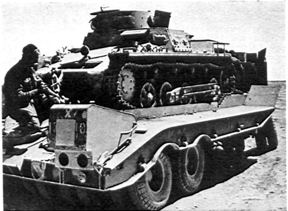
Pz. Kw. I tanks have five spoked bogie wheels on either side (the last four being connected by an outside girder) and four track support rollers. Two light machine guns are mounted coaxially in the turret, which has a rounded back, is on the right side of the tank, and has a very low silhouette. A similar vehicle is used as a commander's tank, in which case the hull is built up to form a square, fixed turret (with only one MG) which in turn carries a square cupola. V-8 engines, acting through the front sprockets, drive these tanks up to 32 mph on roads, with a 95-mile radius of action.
