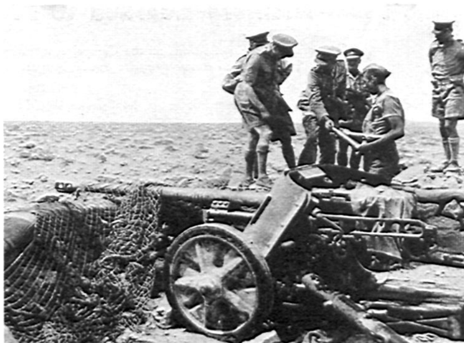
50-mm. antitank guns were issued to the main units of the German Army in the spring of 1941; they are rapidly replacing the older 37's. The carriage has an armor plate shield, muzzle brake, and tubular split trail. Gun (without carriage) weighs 650 lbs., and fires a solid projectile weighing about 4½ lbs. Note the shield's double construction.
