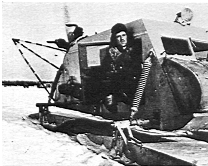
On frozen lakes the Russians widely used sledges driven by air scre??
