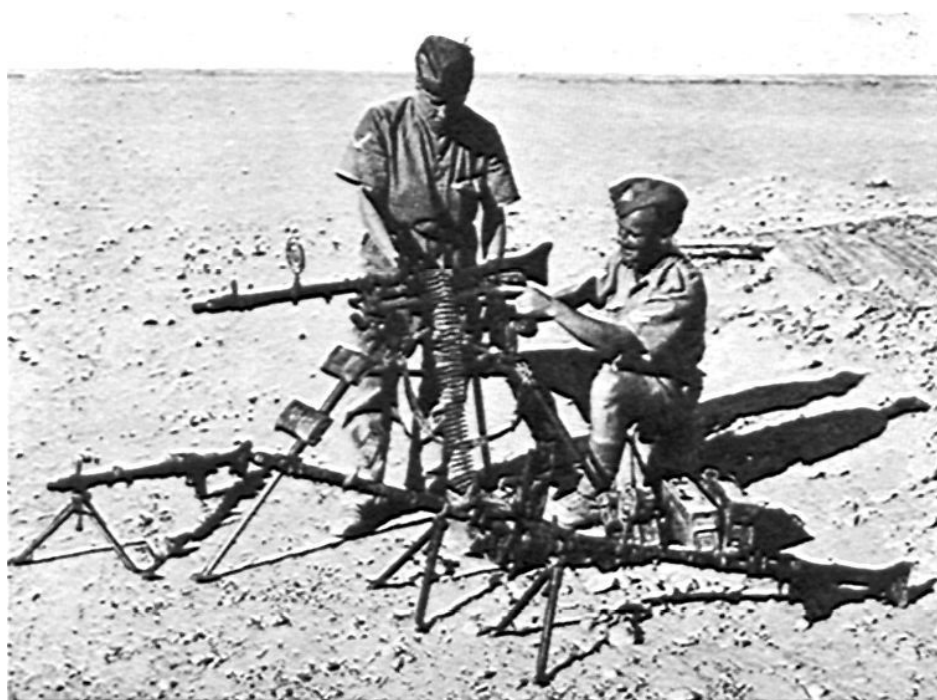
The dual purpose machine gun (MG-34) is now in general use throughout the German Army, replacing both light and heavy models. 7.9-mm. in bore, it weighs only 15½ pounds without mount. Its cyclic rate is 900 rounds per minute, but in practice the maximum rate on bipod is 110-120, on tripod 300-350. The air-cooled barrel must be changed after firing 500 rounds continuously. Metal cartridge belts are extremely flexible, and consist of 10 strips holding 25 each; these parts disconnect when the coupling cartridge is fired. Range: on bipod, 2,200 yards; on tripod and using telescopic sights: 3,800 yards.
