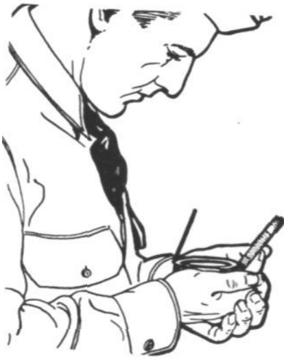
Figure 5. Object sighted is more than 260 mils below operator.
