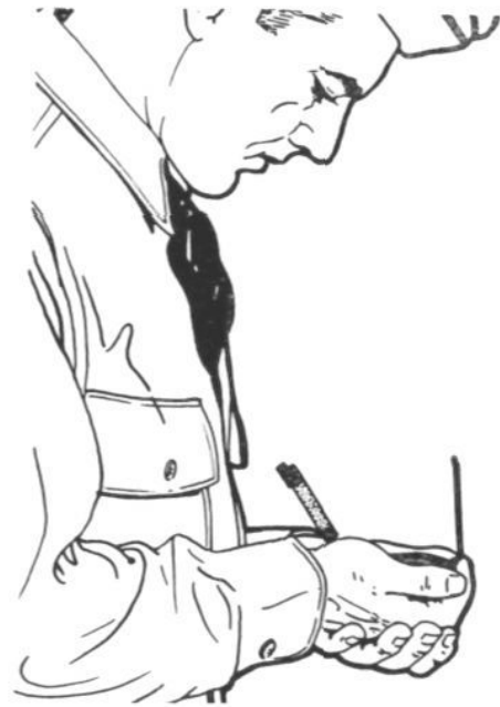
Figure 6. Object sighted is between 800 mils above and 260 mils below operator.
