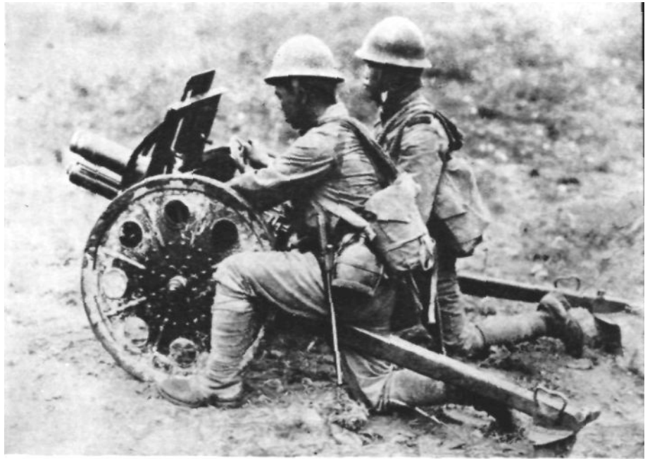
Two Jap gunners man light 70-mm. infantry-accompanying gun. Adequate for its purpose, gun has proven a failure in anti-tank defense. (American Rifleman.)
