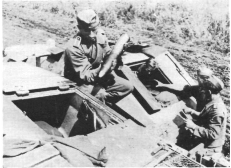
Ammunition being transferred from ammunition tender to armored assault gun. Note thickness of armor on side of assault gun vehicle—about the same as for a light tank. (Acme)
