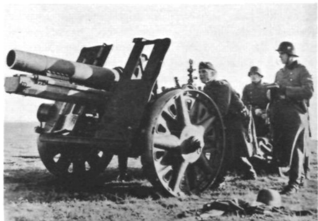
The 75-mm. howitzer (LMW 18) is used as an accompanying weapon by both infantry and cavalry. Although normally drawn by horses or towed by motor, it can be broken into six loads for carrying on packs. Very light in weight, it can be readily manhandled. The box trail permits a 12° traverse. The 14¼-pound shell has an effective radius of 20 yards and a maximum range of 3,900 yards. The rate of fire is very high—15 to 20 rounds per minute.
