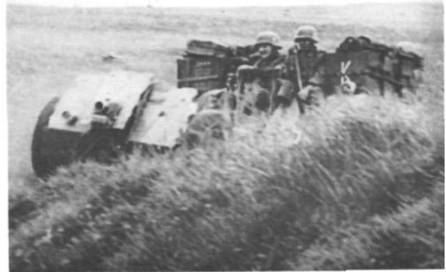
The 150-mm. heavy infantry howitzer (S Inf G 33) is replacing the old 170-mm. trench mortar in all except possibly the Landwehr units. Its weight of 3,300 pounds in action permits considerable manhandling. The box trail allows a 6° traverse and an elevation of some 80°. Rate of fire is around four rounds per minute. Five charges are available, and two projectiles. The 80-pound shell has a range of 6,000 yards, but the 31.8-pound one reaches twice as far. (Acme photo.)
