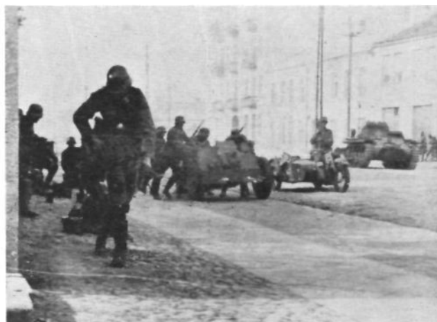
An infantry 75-mm. howitzer is being brought into position. This particular weapon is part of the motorized rifle brigade of a Panzer Division, as indicated by its rubber tires for towing behind a truck. The normal infantry howitzers are not so provided, as they are designed to be drawn by horses. A light tank appears in the right background. The motorcycle with sidecar is furnished for messenger service in all units. (Signal Corps photo.)
