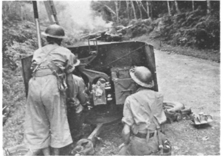
An incautious Jap tank-attack down a road loses three tanks, after they are slowed by hasty block visible above the gun-shield. Note the gun's base-plate for quick all-around fire; the sight projecting above the shield; and the observation ladder at left. The shield appears to be amply large, but thin. (Acme photo)
