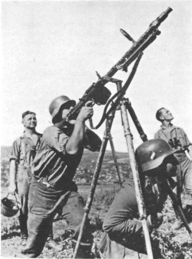
The German dual-purpose MG-34 is rapidly replacing all other machine guns. For ground fire, it uses an extremely flexible metal belt of 10 strips, each holding 25 cartridges. These strips are disconnected when the cartridge joining them is fired. Caliber: 7.9-mm. Maximum range: on bipod, 2,200 yards; on tripod and using telescopic sight, 3,800 yards. Weight without mount: 15½ pounds. (Dever from Black Star.)
