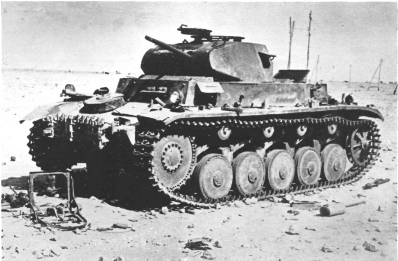
The Pz. Kw. II, standard light (9 tons) German tank. The 3-man crew, protected by 15-mm. armor plate, is armed with a 20-mm. heavy machine gun and one light machine gun in roller type mounting. Maximum road speed is 28 mph; radius of action. 125 miles. Large quantities of these tanks (which are readily convertible to flame-throwers) have been made. The suspension wheels resemble those on our old Christie vehicles. General appearance of the Pz. Kw. II: wide track base, very low silhouette, streamlined.
