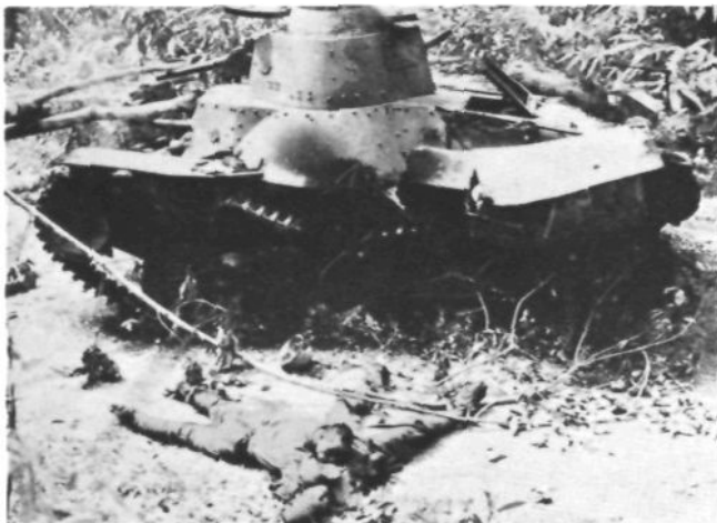
This Jap tankette M2595 (1935) failed to get down the road. Hampered by the road-block, it was destroyed before it could effectively use the 37-mm. turret gun or its machine guns. Its riveted armor, about 1/2-inch thick, was quite insufficient. The block prevented use of its 22 m.p.h. speed. (Acme photo)
