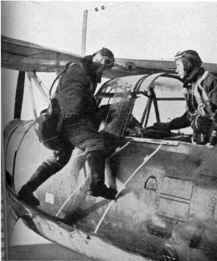
Henschel Hs 126, short-range reconnaissance plane used for photographic missions and to observe for artillery.
