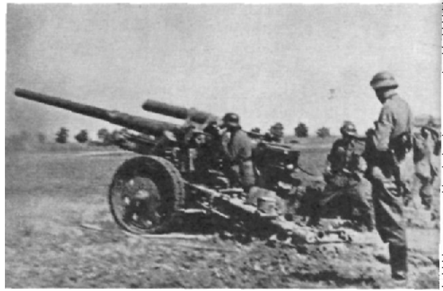
German 105-mm. gun, the long-range weapon which so often interfered with French deployment during a meeting engagement or harassed them during a pursuit. Frequently used for counterbattery. Range about 20,000 yards.
