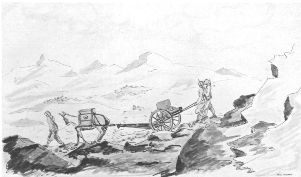
75-mm, gun descending a mountain trail. Note ropes attached to axle's ends.
