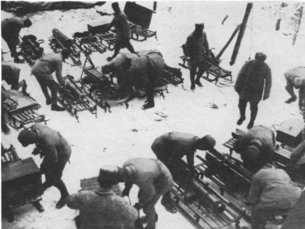
German army winter maneuvers. Packing artillery on sleighs. One sled carries the tube (a 105), one carries cradle, another the trail, and so on. At least six sleighs per weapon seem to be required. (Press Association.)
