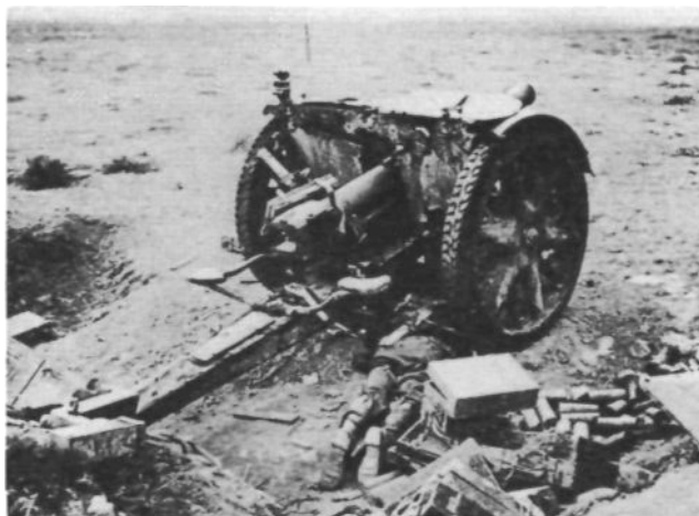
An unprotected field piece is cold meat for the tanks. Here is an Italian howitzer with one of the crew lying dead beside the abandoned piece. Note the German type magnesium wheels and the puncture-proof tires; the latter are a necessity in the desert. (Acme photo.)
