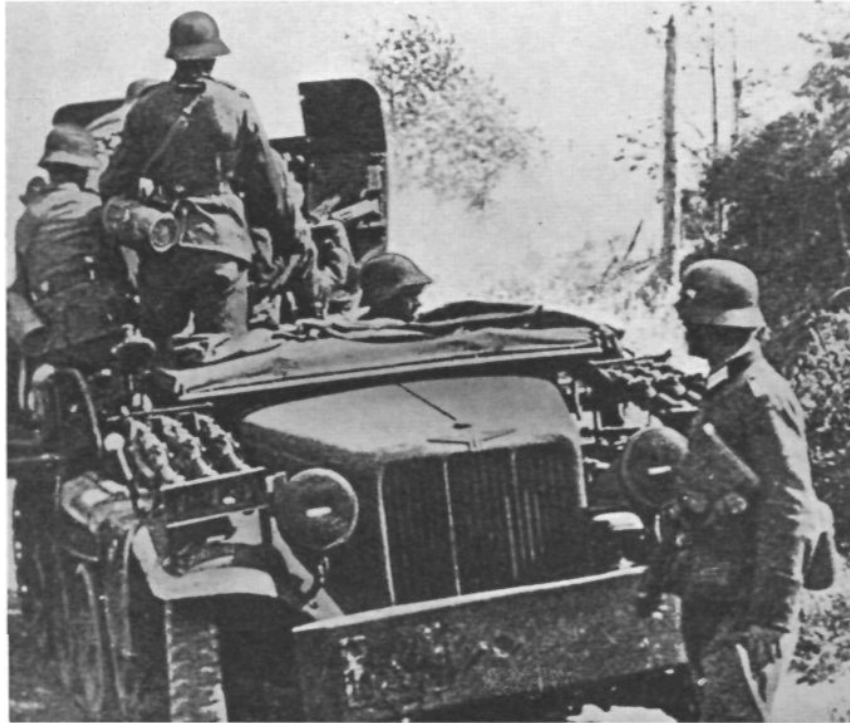
German self-propelled howitzer in action in Russia. These weapons represent a development in artillery materiel which is coming into more and more prominence as the war continues. The advantage of such a weapon is that it gives instant support to advance elements, whereas ordinary towed artillery usually must sit for hours in column on the road waiting to get into action, only to find that its supported infantry has entrucked and is already out of range. (Acme Photo.)
