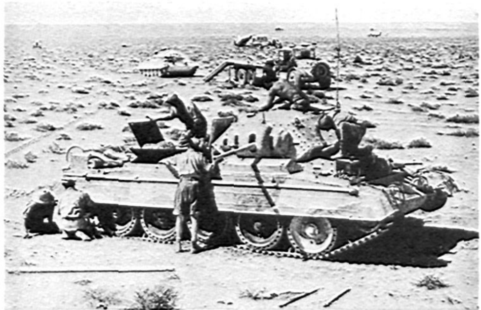
Quick recovery and repair of damaged tanks during (or immediately after) a battle is of prime importance. Desert repair shops must be well dispersed to form an unprofitable target from the air.
