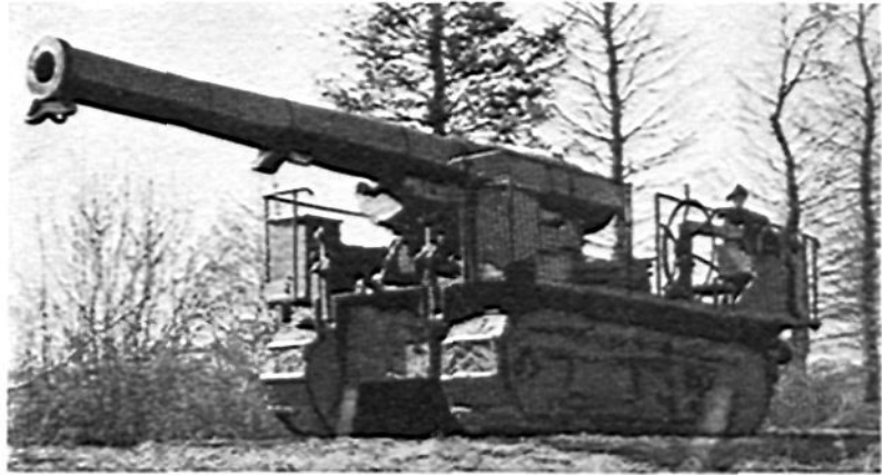
Among the varied types of French artillery was this 194-mm. gun on self-propelled mount (track-laying).
