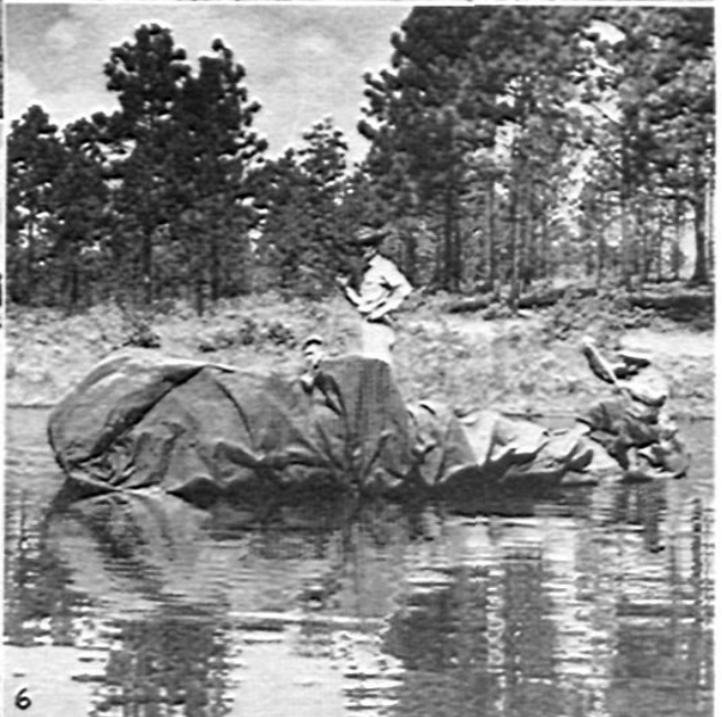
Figure 2—Get tarp mostly afloat, and roll howitzer on while men hold back on edges of tarp.
