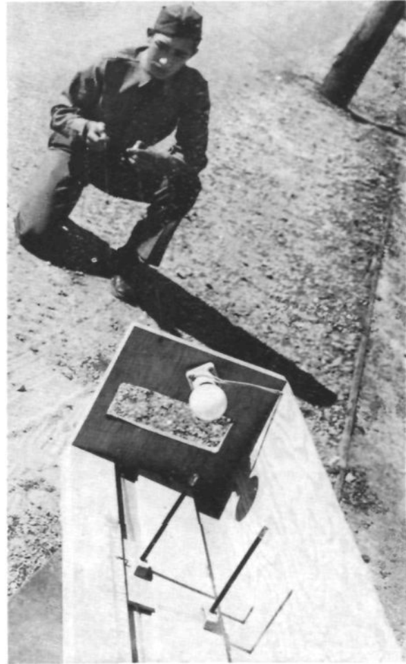
Figure 2: The depth perception test, No. 4. Distance, box to man, 20 feet. The testee holds "reins" by which he controls the movable rod (nearer light).
