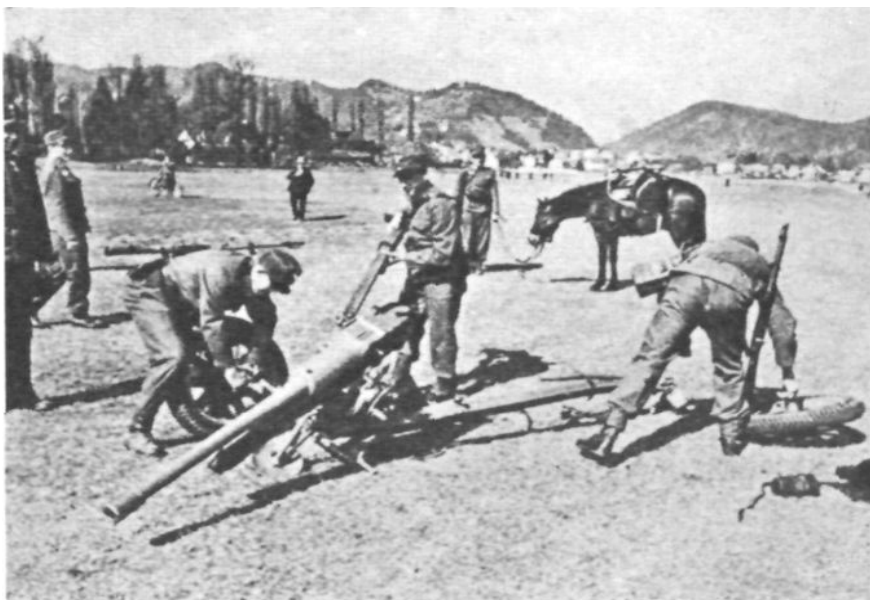
German mountain troops during training exercises just before the outbreak of the war. These pictures show that these units are equipped with an antitank gun which can be towed or packed. It is useful also for airborne troops. This "Pak" is a 47-mm. It has an elevation of 55°, traverse 45°, weighs 517 lbs. in position, muzzle velocity 1900 f/s, range 9000 yds.
