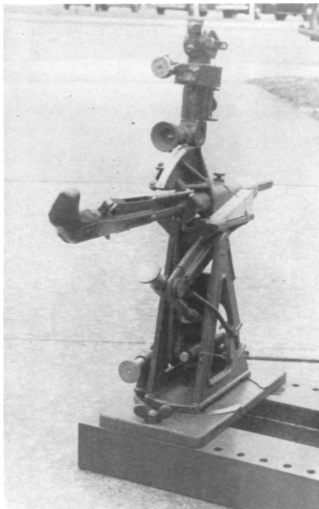
Number Four: note use of springs to eliminate lost motion.
