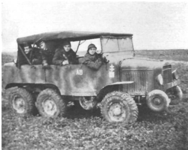
Laffly artillery tractor, used by 71st FA. It is powered by a Hotchkiss engine, 100 HP., used as reconnaissance vehicle and prime mover. Photo by Leo Framery.
