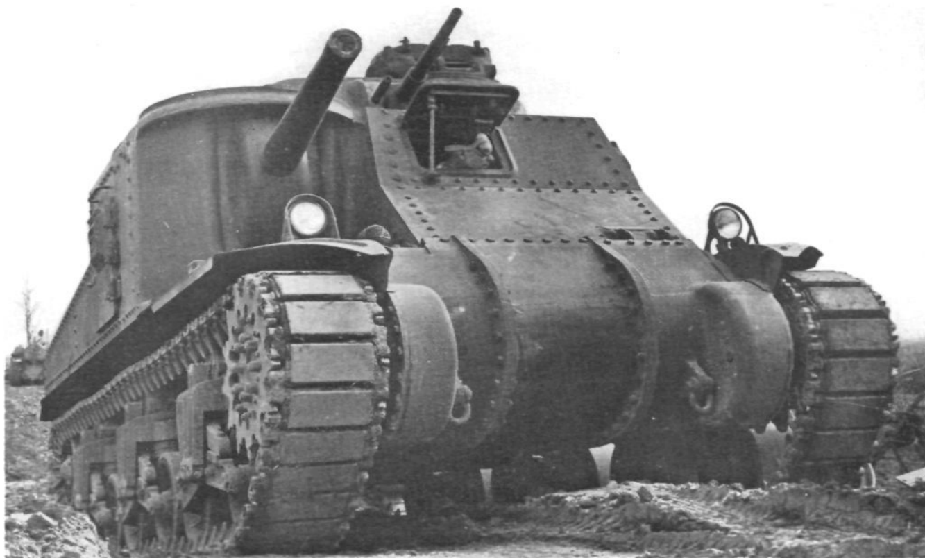
The 75-mm. cannon makes the new medium tank M3 a formidable weapon
