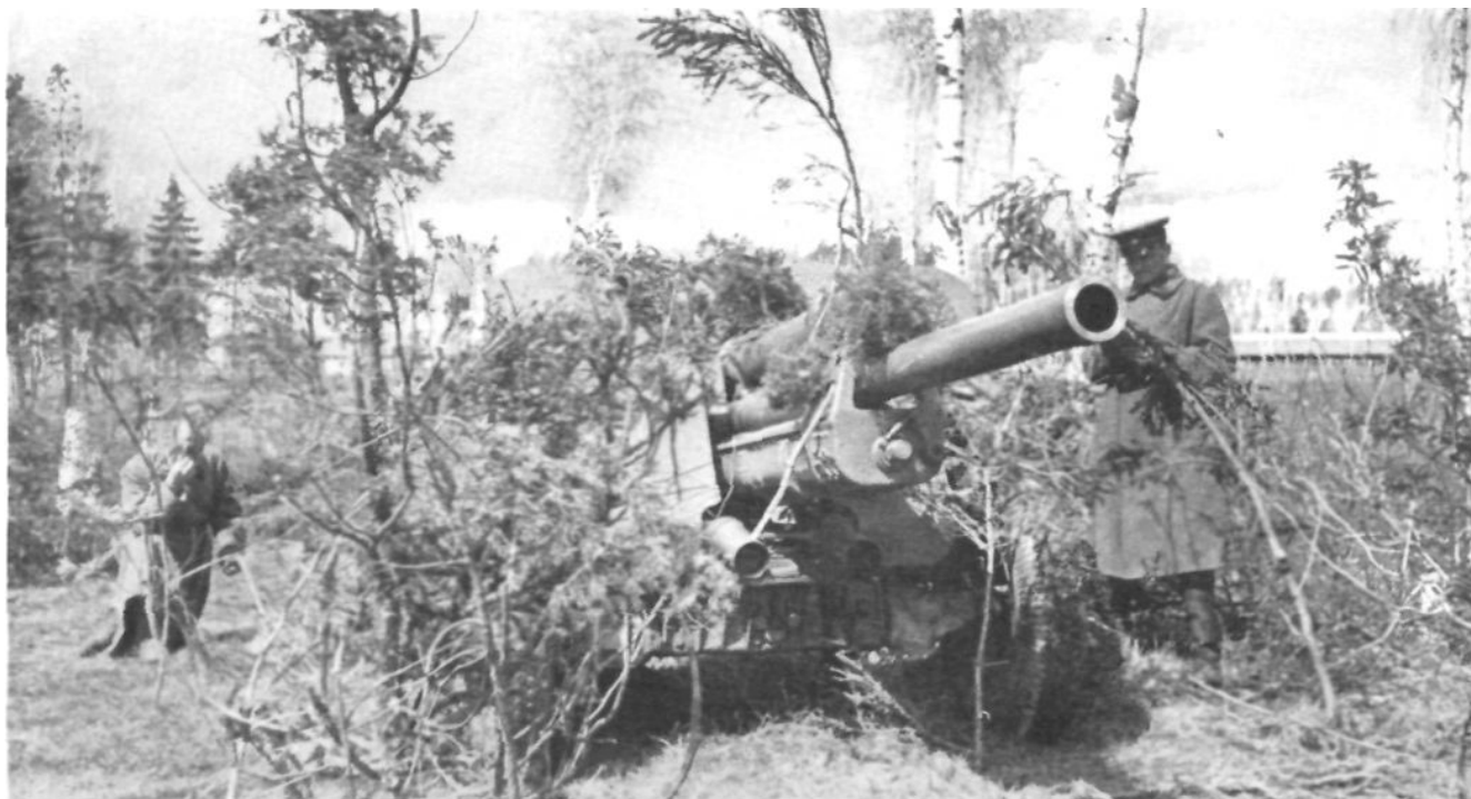
A Russian field piece in camouflaged position during training exercises in 1941. Note the German type shield; the equilibrators under the recoil mechanism; the heavy axle; the split trail. This is the late model weapon, probably a 76-mm modified Bofors type, or possibly a 122-mm gun-howitzer. Note the firs and birches, common to the northern latitudes.
