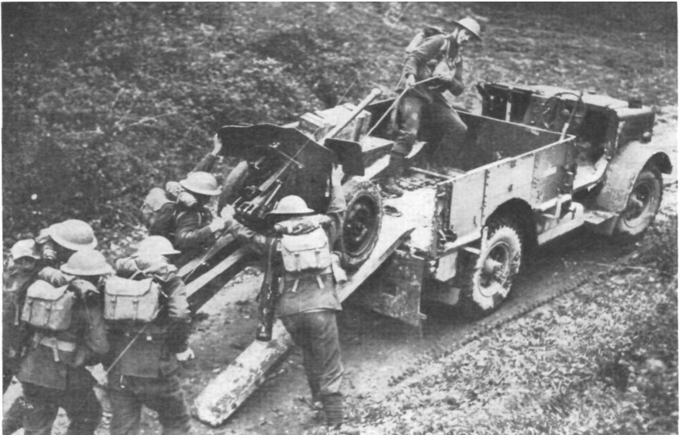
British antitank regiments, which are a part of the divisional artillery, frequently portee some of their weapons. In the Russo-German War both sides are carrying guns in trucks, and firing them therefrom, as tank chasers.
