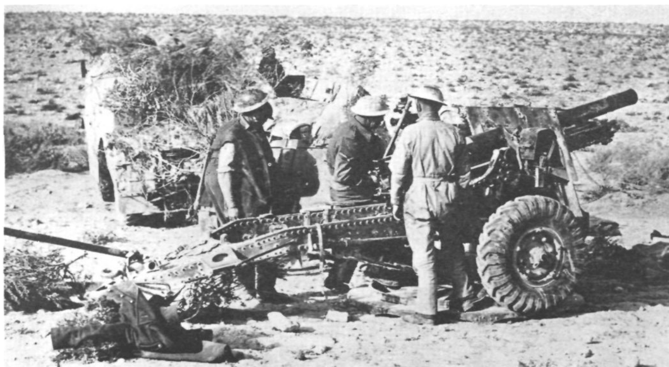
British guns being brought into position on the side of Tobruk prior to taking part in a mass bombardment. Note the metal platform under the piece, which gives 360° traverse.
