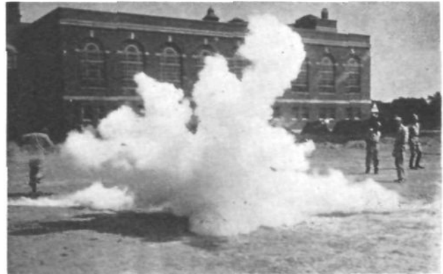
Picture of the explosion of one of the lime bombs, developed to simulate the bursting of an artillery shell. After the smoke has cleared, lime dust will be distributed over the ground to the extent of the smoke shown.
