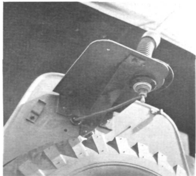
View showing details of mounting at base of antenna
