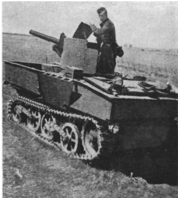
German tank "chaser." Reproduced from the Spanish army review "Ejercito," this shows that the Germans are making use of captured vehicles and weapons to construct armored self-propelled antitank guns which they apparently will use in large numbers in their new Panzer divisions. Illustrated here is a captured British Bren machine gun carrier in which is mounted what may be a 47-mm. or larger antitank gun. The resulting vehicle is not exactly a tank, but it carries light armor for protection of the crew, while the gun shield furnishes protection against tank fire. Note that the vehicle has low silhouette, and that the gunner will have good visibility for all-round fire. Previous photographs reproduced in THE FIELD ARTILLERY JOURNAL indicate that the Germans will employ their own light tank chassis, with the turret removed, for similar purposes.
