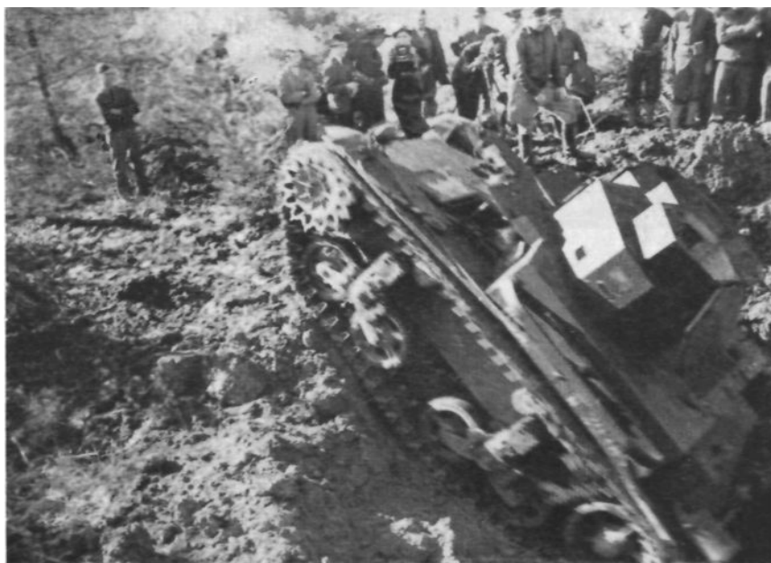
Fig. 8—Tank fails to pass crater made by 150 lbs. of TNT used in variation on standard method.
