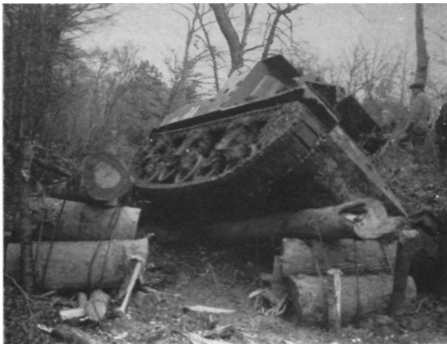
Figure 5—Medium tanks bellied on saw-horse type obstacle.
