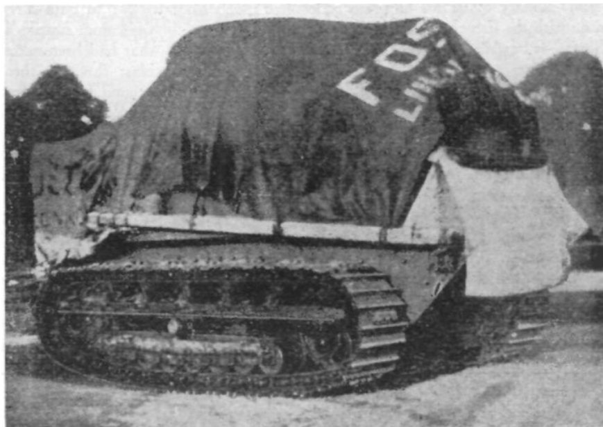
"Little Willie," the experimental—and unsuccessful—model for the first tank.
