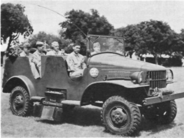
Fig. 1. Right side of the radio truck, showing 12-volt storage battery with battery case opened.
