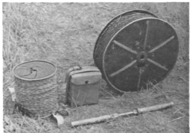
Showing relative size of commercial spool of W-130, ordinary telephone, and DR-4 Drum. The spool holds one-half mile and weighs about 25 pounds.
