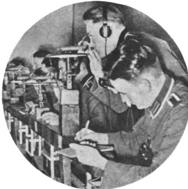
Exercises in the use of flash-ranging instruments for night firing. The students of the military school sit in a darkened room in front of a sand box containing an electric lamp which emits flashes resembling lightning from time to time. These represent the flashes of the enemy's guns. They first practice locating the enemy batteries by intersection in the school room, and go out into the field later.
