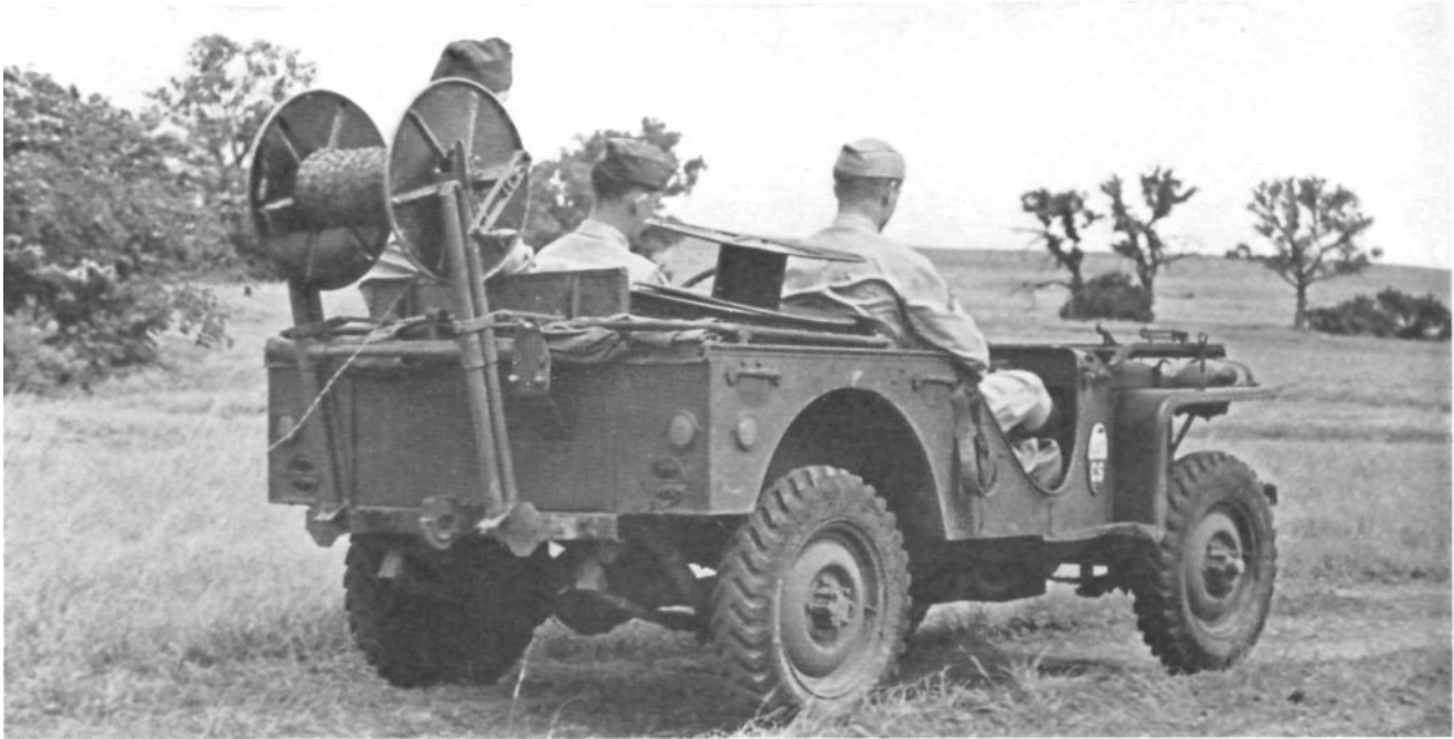
Quarter ton 4x4 bantam car with DR-5 drum mounted on RL-31 frame attached. The DR-5 drum carries two miles of W-130. Five miles can be carried.
