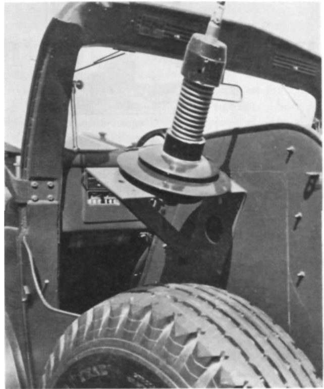
Fig. 2. Close-up view of mast bracket MP-41.
