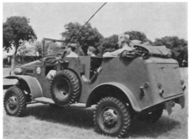
Fig. 3. Improvised mast bracket, constructed at F.A. School, mounted on radio truck.
