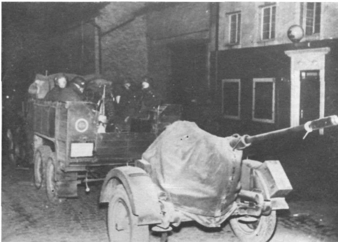
German 20-mm. Flak passing through French village at night. Used for close defense of columns or positions, against low-flying aircraft. Note white markings on rear of truck, for guidance of following vehicle.
