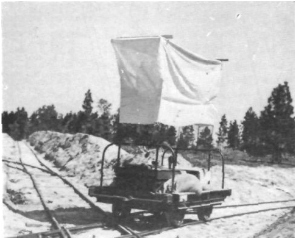
Commercial motor car, unmodified, used as target carrier.
