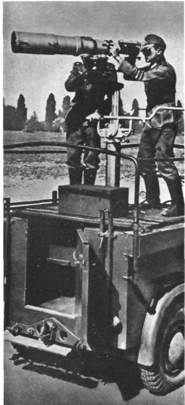
German long-range camera, used for observing artillery fire and making photos of distant target areas. Has taken clear photos at ranges up to 45 kilometers.
