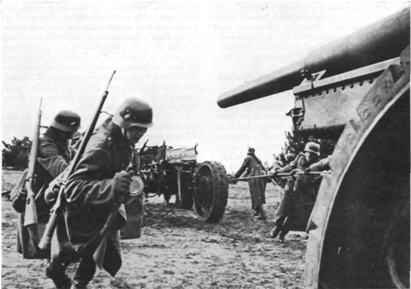
Heavy German howitzer (15-cm. or 21-cm.) going into position. The weapon is transported in two loads. Here we see the cannoneers dragging up the carriage transport wagon to slide the tube on to the cradle.
