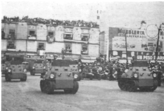
The Mexican Tank Corps passes in review. The vehicles are Marmon-Herrington light tanks powered with Ford engines and carrying two light machine guns.
