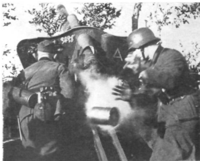
German 105-mm. howitzer in action Note base deflection chalked on shield
