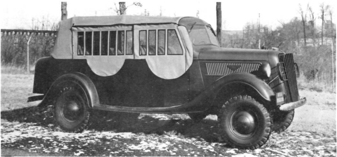
Pilot model of command car. The production vehicles (Dodge) embody certain modifications and improvements
