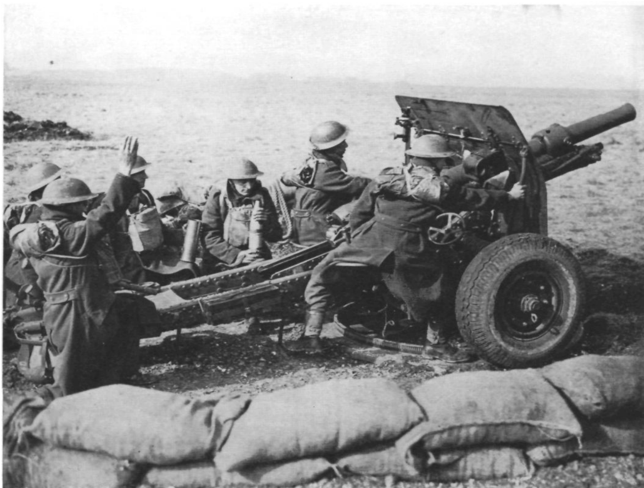
British divisional field piece. Note circular platform for use in firing at moving targets.
