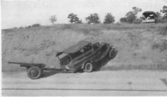
GUN AND TRUCK ASCENDING A NEARLY VERTICAL BANK WITH THE AID OF THE UNDERSLUNG WINCH
