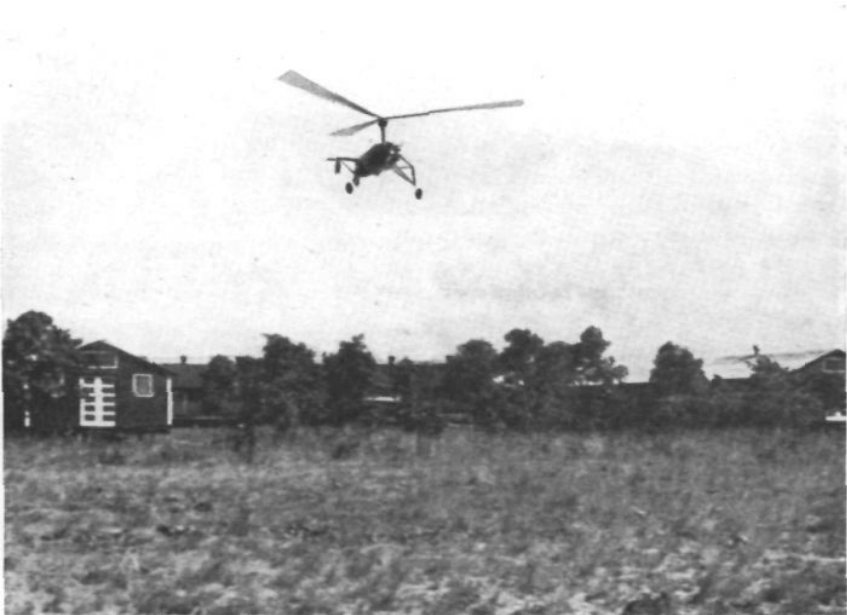
THE AUTOGIRO IN FLIGHT. NOTE THE CONING OF THE ROTOR BLADES.
