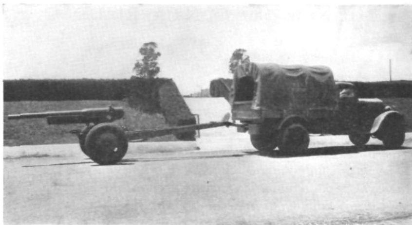
EACH PILOT MODERNIZED CARRIAGE WAS GIVEN ROAD AND CROSS COUNTRY TESTS TOTTALLING OVER 5000 MILES
