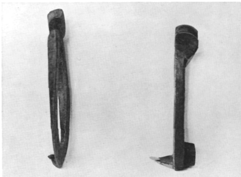
RIGHT VIEW, NEW SHOE, FOR DRAFT ANIMAL MADE UP WITH CAULKS ON HEEL AND TOE
