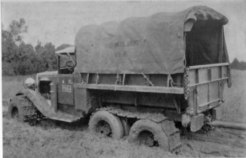
THE LIGHT PRIME MOVER T9, SIX WHEEL, SIX WHEEL DRIVE MARMON HERRING. TON TRUCK, EQUIPPED WITH HIPKINS TRACTION DEVICES, TOWING THE 155MM HOWITZER THROUGH THE MUD COURSE AT ABERDEEN PROVING GROUND.
