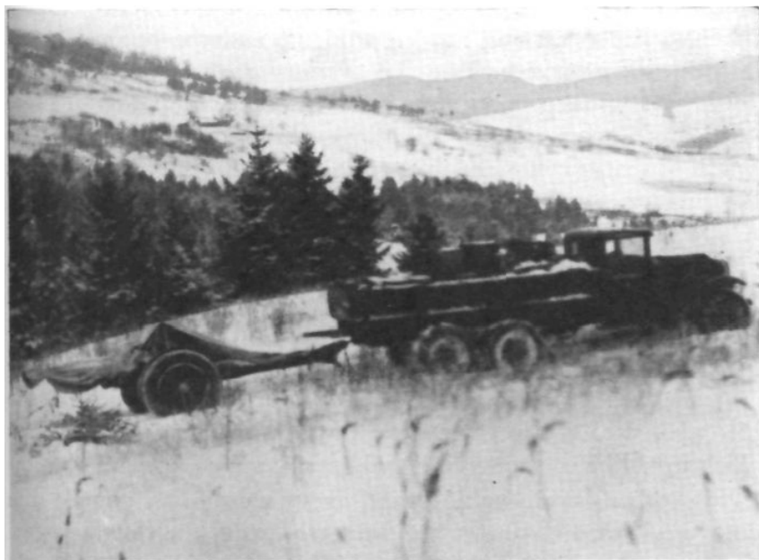
6-WHEEL TRUCK ON OVAL HIPKINS' TRACK TOWING GUN UP STEEP GRADE IN SNOW.
