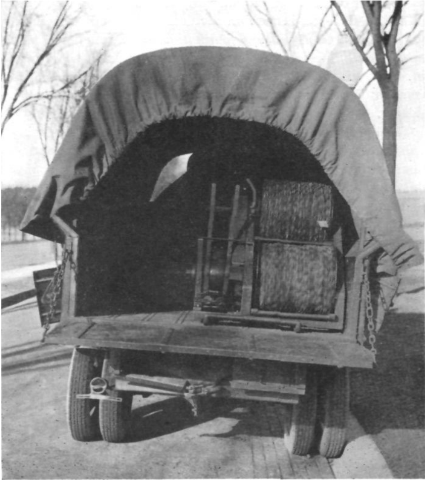
THE REEL RL-26 MAY BE USED IN ANY TRUCK OF THE BATTERY
