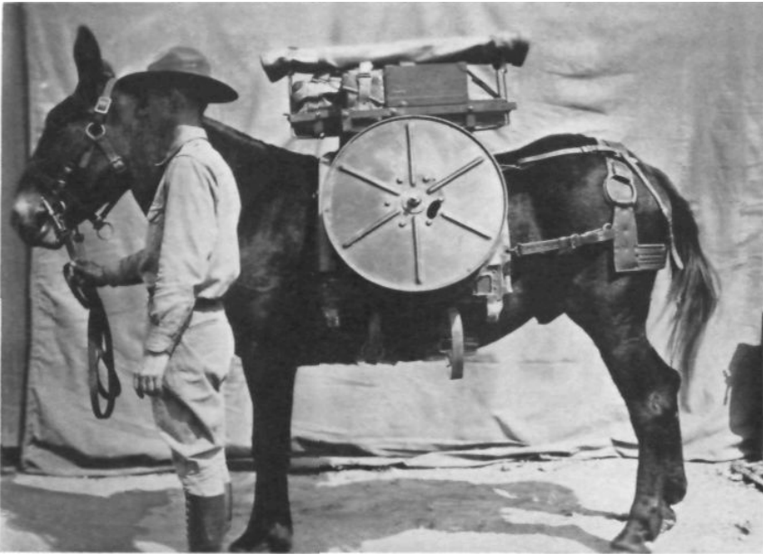
RADIO PACK NO. 2 (COMBINED WIRE AND RADIO PACK FOR LIAISON SECTION, CARRYING SCR NO. 161 RADIO SET AND TWO SPOOLS OF WIRE.)
