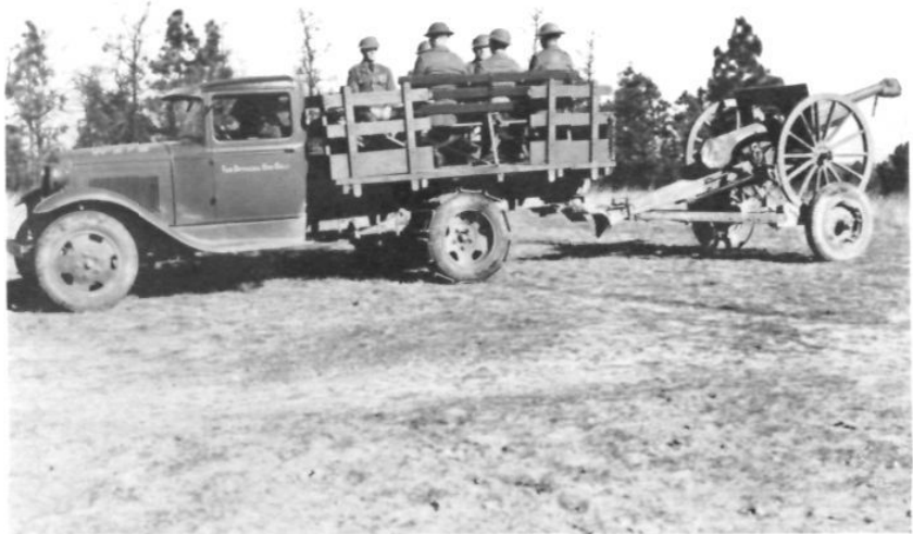
FIGURE 3.—DYNAMOMETER TEST OF A FORD TRUCK WITH SUB-TRANSMISSION AND HIPKINS TRACKS. TOTAL WEIGHT OF GUN AND DYNAMOMETER, APPROXIMATELY 30,000 POUNDS
