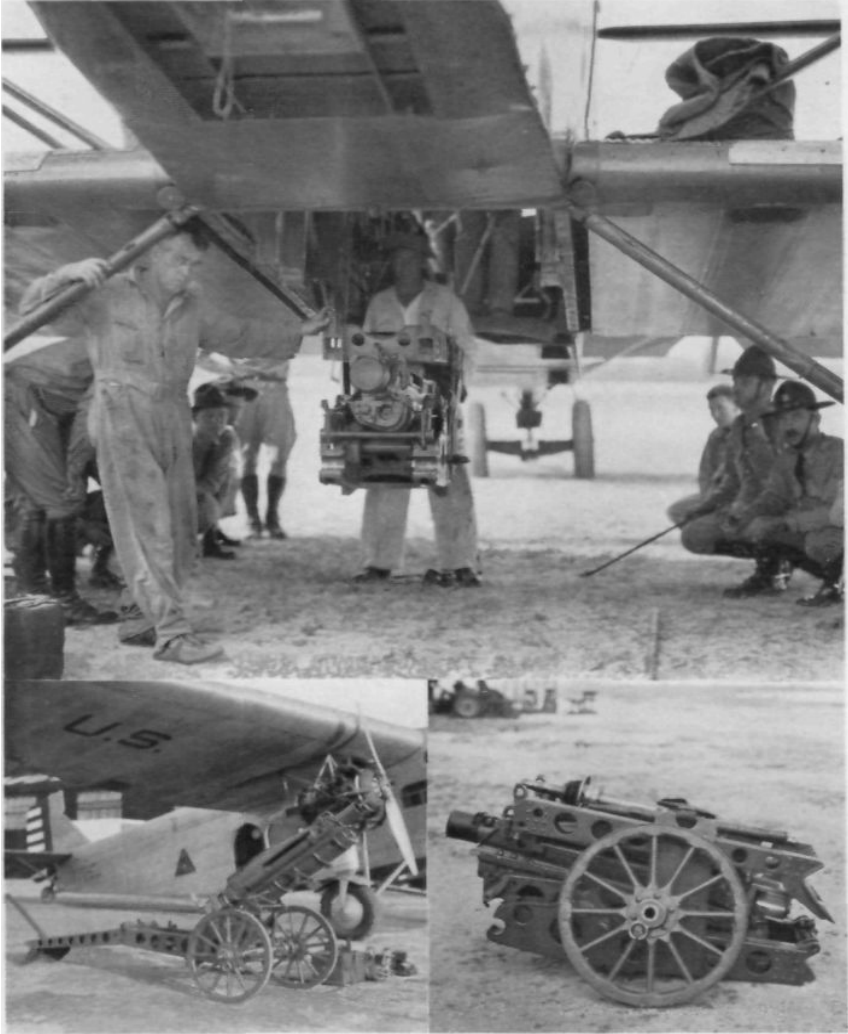
ABOVE: 75MM. HOWITZER BEING LIFTED INTO KEYSTONE BOMBER LOWER LEFT: FORD MONOPLANE ABOUT TO TAKE ON A PACK HOWITZER LOWER RIGHT: THE NEW PACK HOWITZER PACKED FOR FLYING
