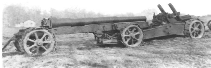
FIGURE 5. 155MM. GUN, 8" HOWITZER CARRIAGE, M1920E
