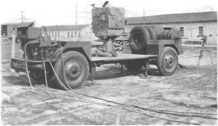
DIRECTOR M2 MOUNTED ON INSTRUMENT TRAILER NOTE POWER PLANT AND REELS FOR TRANSMISSION CABLES
