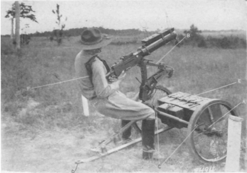
FIGURE No. 1: A—WHEELS DETACHABLE IN THREE SECONDS FOR GROUND USE. B—ANTI-AIRCRAFT ADAPTER FOLDS UP IN FIVE SECTIONS. C—TRIPOD CAN BE REMOVED INSTANTLY FROM MOUNT. D—LUNETTE WHICH ENABLES GUN AND MOUNT TO BE TRAILED IN ANTI-AIRCRAFT FIRING POSITION, LOADED E—AMMUNITION, RESERVE LOAD. F—TANK SHOULDER REST. (THIS IS UPSIDE DOWN TO NORMAL TANK USAGE.
