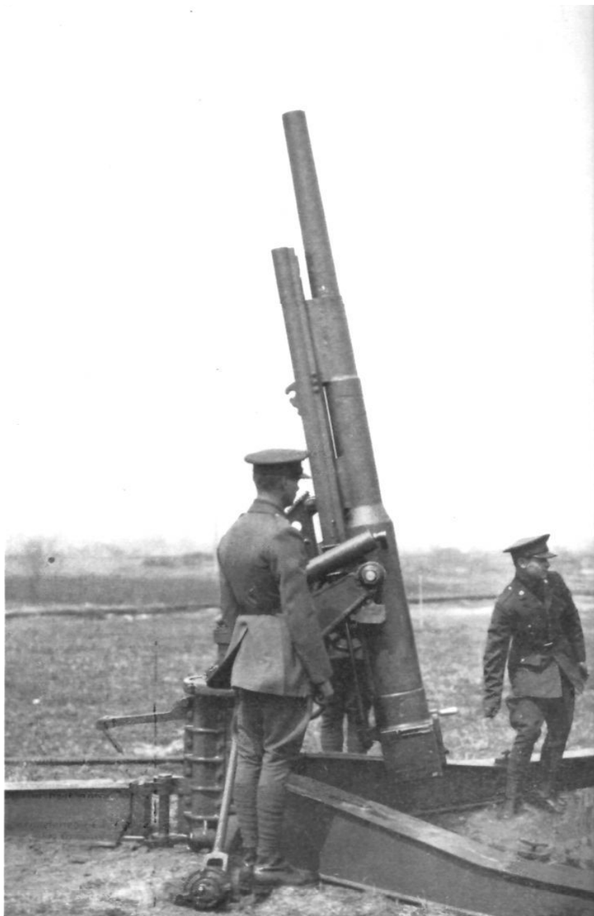
T2 DIVISION ARTILLERY MOUNT GUN AT FULL RECOIL, 80° ELEVATION
