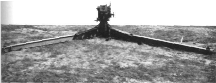
FIG. 2. REAR VIEW OF T2 MOUNT IN POSITION FOR ALL-AROUND FIRE
