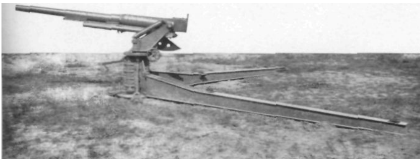
FIG. 6. IN POSITION FOR LIMITED TRAVERSE, USING ONLY TWO OUTRIGGERS
