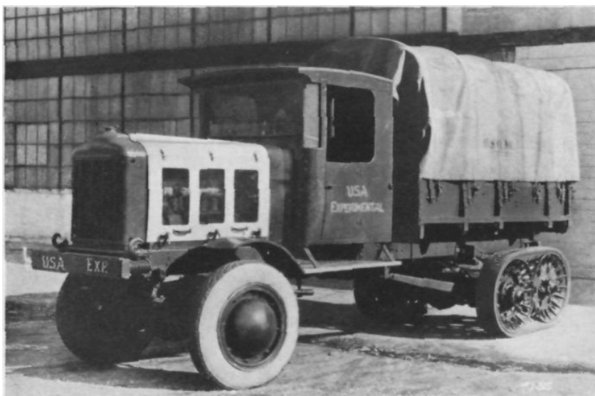
ARMY EXPERIMENTAL TRUCK WITH PNEUMATIC TIRES IN FRONT AND RUBBER TREAD IN REAR
