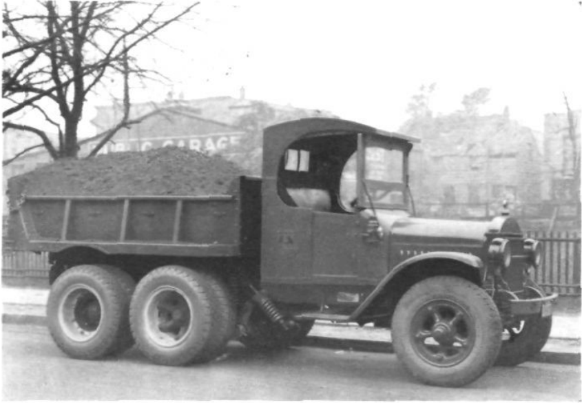
MACK DUAL PNEUMATIC TRUCK DESIGNED FOR SPEED WITH HEAVY LOADS
