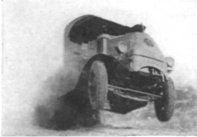
LEFT—MACK TRUCK WITH CHRISTIE CRAWLER CLIMBING OUT OF EXCAVATION WITH SPECIAL LEVER CONTROL FOR STEERING WHEN FRONT WHEELS LEAVE GROUND. RIGHT—AN 8-TON LOAD GOING THROUGH A SWAMP IN WINTER
