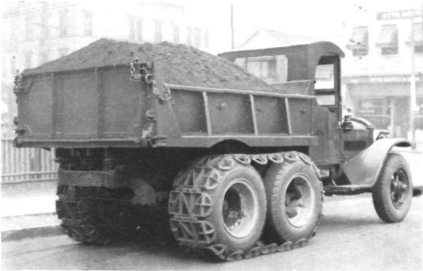
SAME TRUCK EQUIPPED WITH NEW-TYPE TREADS FROM WHICH DRIVING ROLLERS AND TUGS HAVE BEEN ELIMINATED
