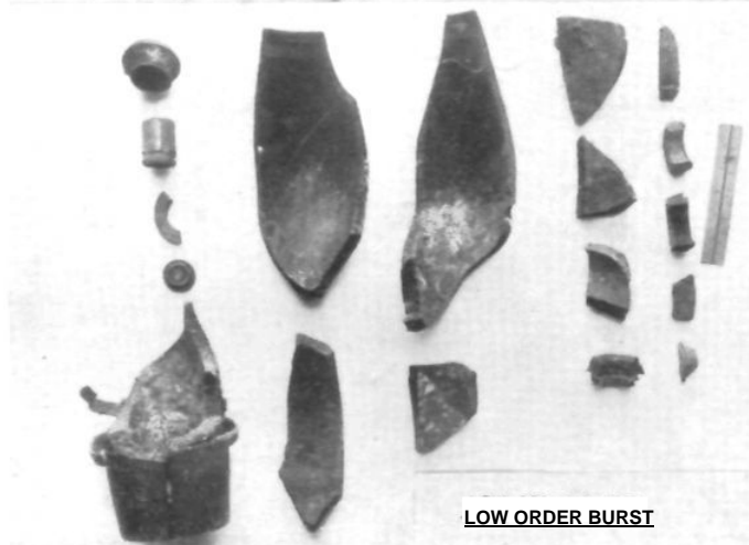
CHARACTERISTIC EFFECTS OF HIGH ORDER DETONATION AND LOW ORDER BURST—4.7-INCH HIGH EXPLOSIVE SHELL.
