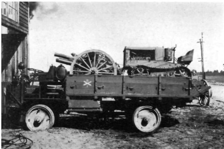
HOLT 2-TON TRACTOR AND 75-MM MODEL 1916 GUN IN F. W. D. TRUCK (NOT MODIFIED)
