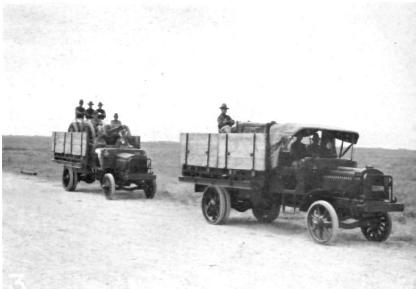
SECTION READY TO MOVE, 3-INCH GUN AND CAISSON WITH 2-TON TRACTOR LOADED ON TWO TRUCKS
