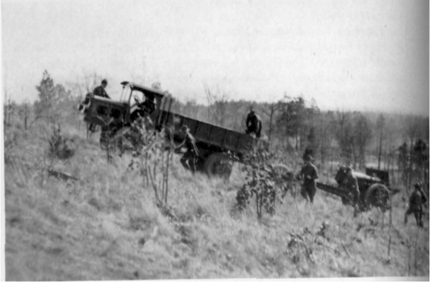
COLEMAN TRUCK LOADED WITH THREE TONS OF DIRT AND TOWING A 155-MM. HOWITZER ASCENDING 18° SLOPE
