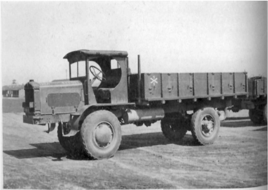
COLEMAN 5-TON TRUCK—SIX CYLINDER—PNEUMATIC TIRES
