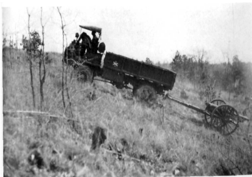
F. W. D. TRUCK LOADED WITH ONE AND ONE HALF TONS OF DIRT AND TOWING A 3-INCH GUN ASCENDING AN 18° SLOPE
