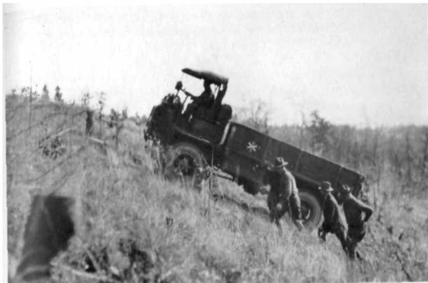
F. W. D. TRUCK LOADED WITH THREE TONS OF DIRT ASCENDING 18° SLOPE
