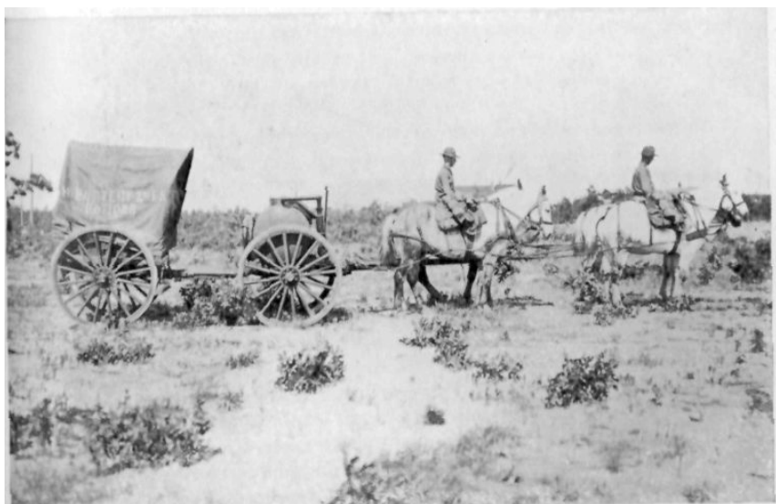
TWO-AXLE LOAD PROPOSED TO REPLACE THE TWO ONE-AXLE LOADS AUTHORIZED AS BATTERY EQUIPMENT
