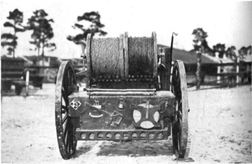
BATTERY REEL MODIFIED TO CARRY EXTRA REELS
