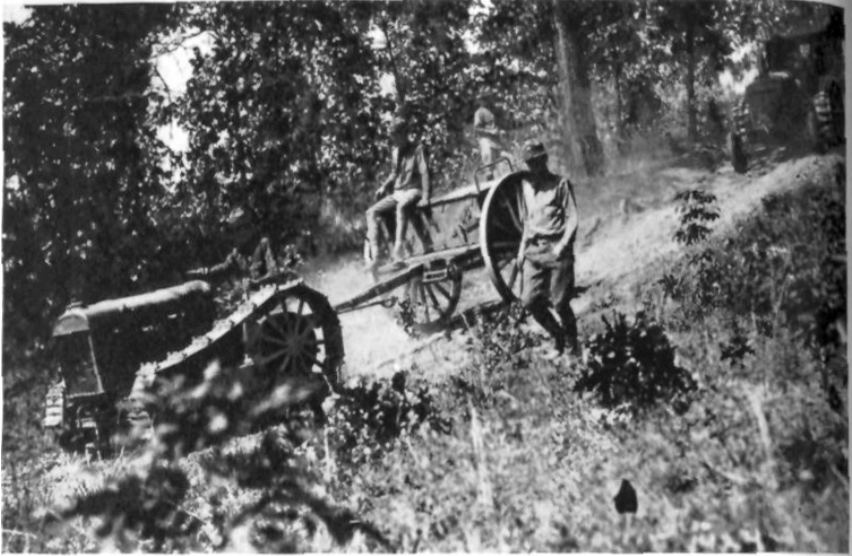
FORDSON TRACTORS WITH ADAPTERS—FULL-CRAWLER ON THE LEFT, HADFIELD-PENFIELD ON THE RIGHT
