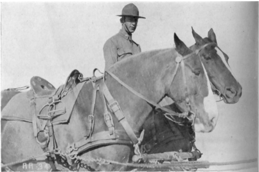
THE YOKE LYING ON THE SUPPORTED POLE
