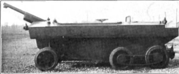
75-MM. GUN CARRIAGE, CHRISTIE COMBINED WHEEL, TRACK-LAYING AND SELF-PROPELLED FLOATING TYPE
