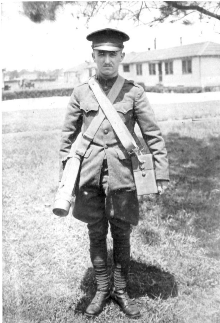
FIG. 4.—SCR-77-A SET. METHOD OF CARRYING WHEN EMPLOYING TWO MEN This photograph shows loop in its carrying bag and one BB-41 battery
