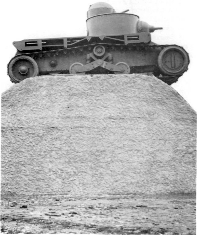
MEDIUM TANK (CHRISTIE TYPE) Going up and down 45° and 35° slopes.
