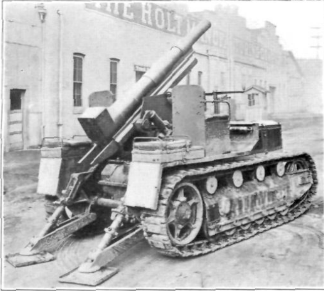
CATERPILLAR MOUNT FOR 75-MM. GUN AND 105-MM. HOWITZER
