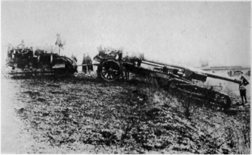
155 MM. G. P. F. GUN, WITH ONE 10-TON ARTILLERY TRACTOR ATTACHED, AT BOTTOM OF 30° GRADE UNABLE TO PROCEED FURTHER. TWO 10-TON ARTILLERY TRACTORS HITCHED IN PARALLEL PULLED GUN UP GRADE.
