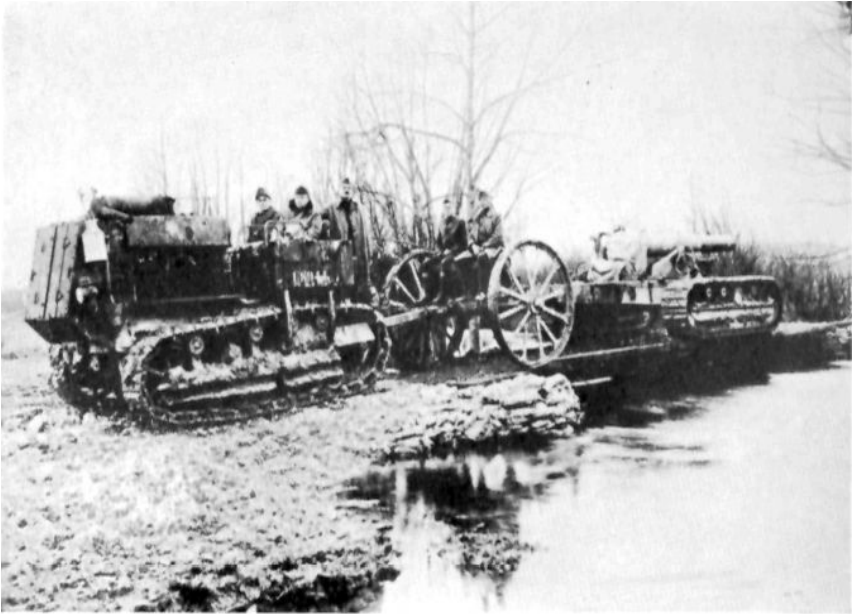
TRAILING 8-INCH HOWITZER ACROSS VERY NARROW BRIDGE, SHOWING TRACKS ON HOWITZER EXTENDING OVER EACH EDGE ABOUT 10 INCHES.
