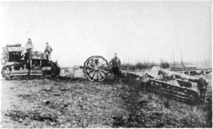
8-INCH HOWITZER, WITH CATERPILLAR ATTACHMENT UNITS, BEING PULLED UP SHORT GRADE OF APPROXIMATELY 30° WITH ONE 10-TON ARTILLERY TRACTOR-HOWITZER AT BOTTOM OF GRADE.
