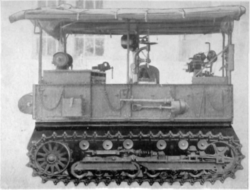
PHOTOGRAPH NO. 5. ARTILLERY REPAIR TRAILER CAISSON. (See paragraph 4-g.)
