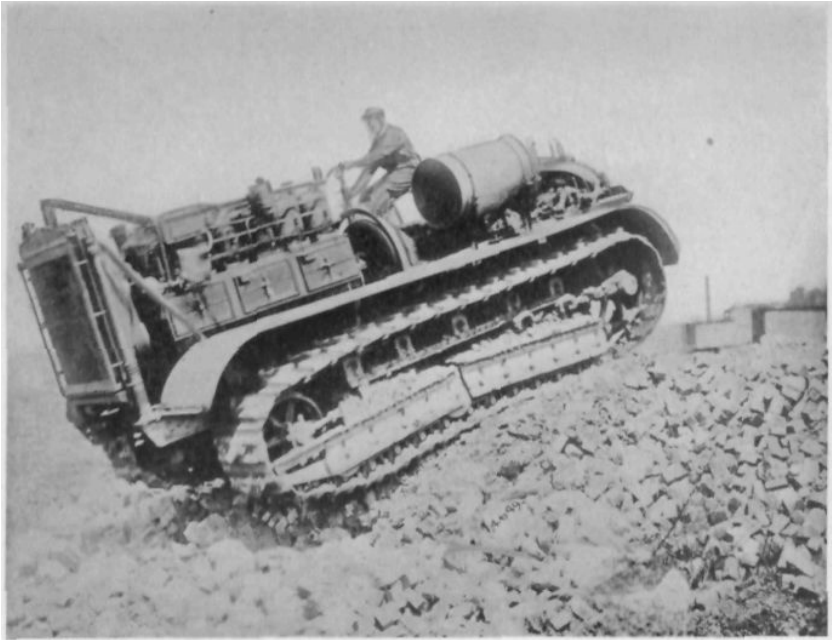
PHOTOGRAPH NO. 15. THE 15-TON ARTILLERY TRACTOR. (See paragraph 8-d.)
