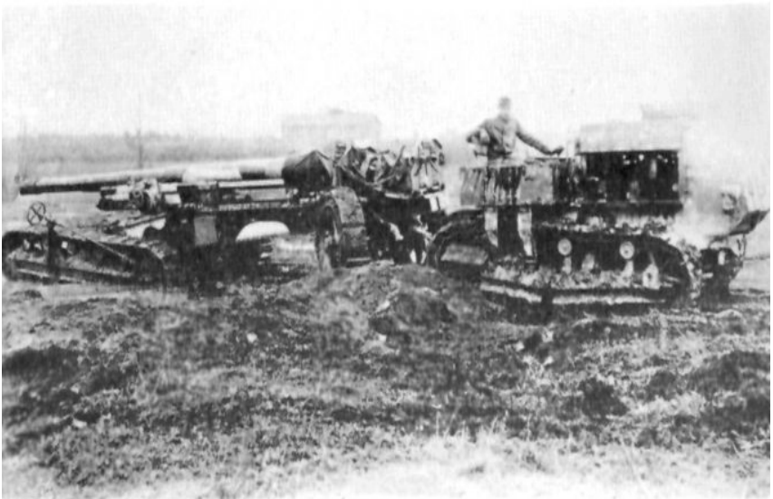
155 MM. G. P. F. GUN EQUIPPED WITH CATERPILLAR ATTACHMENT UNITS AND CATERPILLAR BAND SHOES (CINGOLI) ATTACHED TO FRONT WHEELS TO SUPPORT WEIGHT OF TRAIL SPADES AND HYDRAULIC JACKS.
