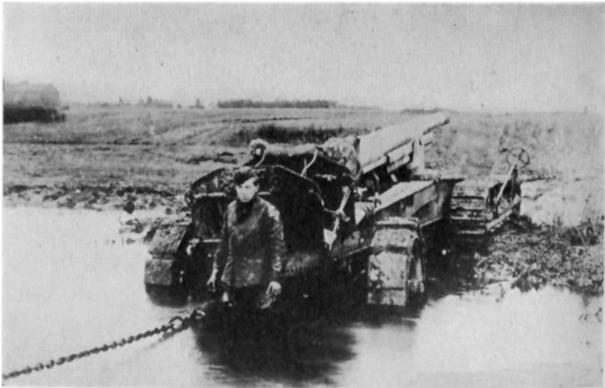
155 G. P. F. GUN IN A POSITION FROM WHICH 20-TON TRACTOR WAS UNABLE TO PROCEED FURTHER DUE TO INABILITY OF TRACTOR TO CLIMB OPPOSITE BANK. PHOTOGRAPH ALSO SHOWS CHAIN CONNECTION BY WHICH GUN WAS PULLED ACROSS STREAM WITH 10-TON ARTILLERY TRACTOR ON OPPOSITE BANK.
