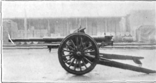
WOODEN MODEL OF 75 MM. GUN ON SPLIT TRAIL CARRIAGE The 105 mm. howitzer will be mounted on same carriage
