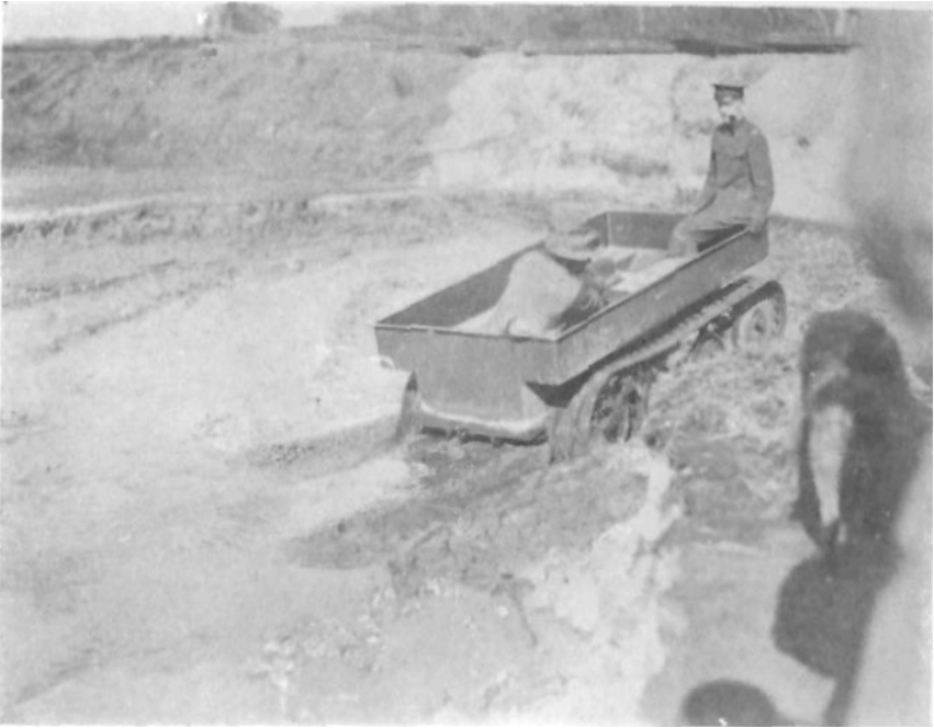
FIG. 5.—RECONNAISSANCE TRACTOR GOING THROUGH QUICKSAND
