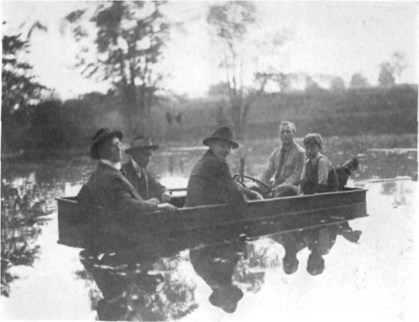
FIG. 3.—RECONNAISSANCE TRACTOR DEMONSTRATING ITS ABILITY TO FLOAT WHEN LOADED
